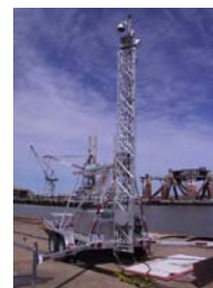
Portable Telescoping Antenna Trailer With Remotely Operated Surveillance Camera
